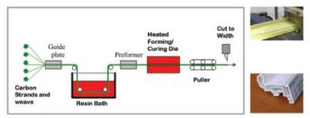
**Pultrusion**: This design uses composite materials in conjunction with a new manufacturing process called 'Pultrusion' to make a vehicle occupancy zone. To raise production numbers and make this chassis even more affordable, one occupancy zone must work in all passenger vehicles in a brand's line-up.
